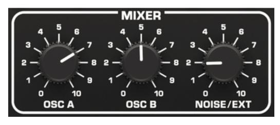
audio input is used, noise is bypassed and this knob sets the level of external signal input to the FILTER.
